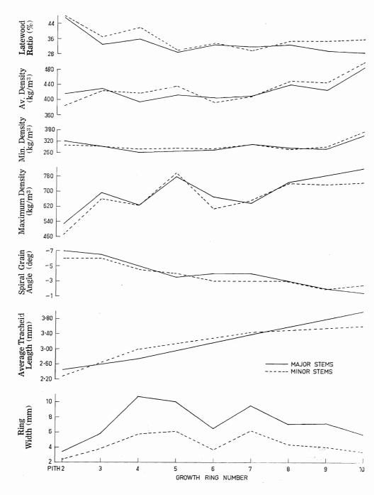
FIG. 3—The variation through successive growth rings from the pith of the mean of ring width, average tracheid length, spiral grain angle, maximum, minimum and average density and latewood ratio for breast high specimens from the major and minor stems of three double-stemmed trees from Blue Range plantation, A.C.T.
