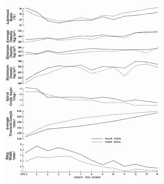
FIG. 2—The variation through successive growth rings from the pith of the mean of ring width, average tracheid length, spiral grain angle, maximum, minimum and average density and latewood ratio for breast high specimens from the major and minor stems of three double-stemmed trees from Kowen plantation, A.C.T.
