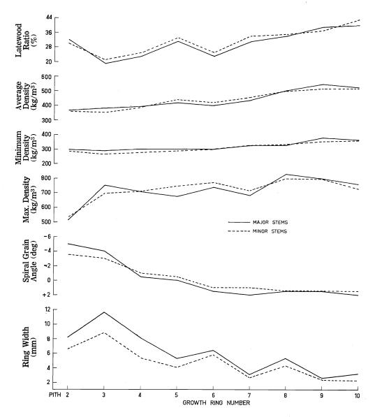
FIG. 1—The variation through successive growth rings from the pith of the mean of ring width, spiral grain angle, maximum, minimum and average density and latewood ratio for breast high specimens from the major and minor stems of three doublestemmed trees from Vanities Crossing plantation, A.C.T.
