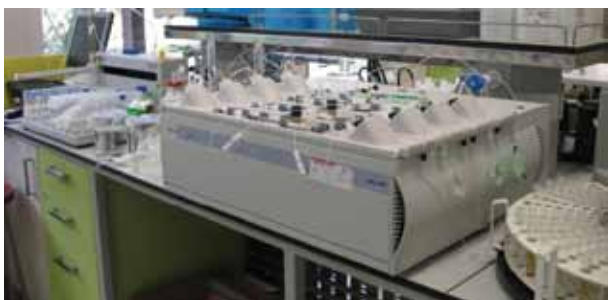
We have invested in a new FIA (Flow Injection Analyser) for nutrient analysis. The FIA is faster and is widely used in other laboratories around the country.
