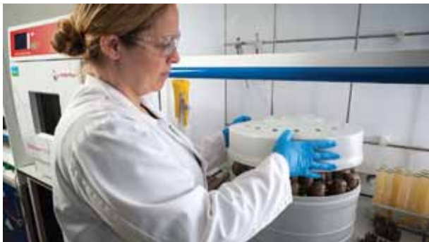
The digester provides more efficient preparation and digestion of samples prior to them being run on instruments.
