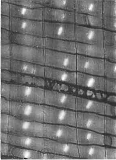
FIG. 5—Stem RLS \times 325 . Ray parenchyma with thin horizontal walls. A ray tracheid lies across the centre.
