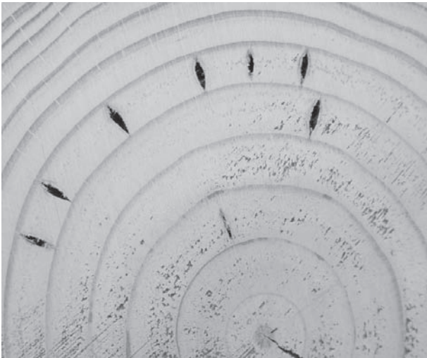
FIGURE 11: Cross section of radiata pine stem showing resinous checking (wet checks) within growth rings.
