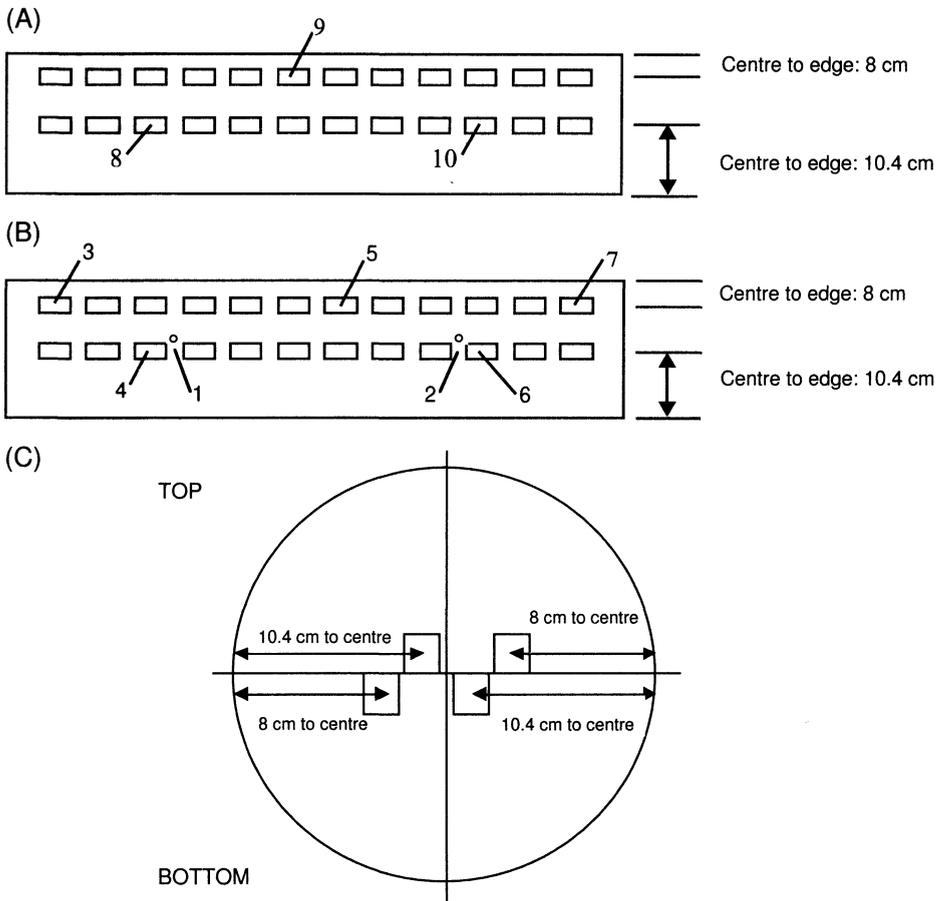
FIG. 1—Schematic longitudinal top (A), bottom (B), and frontal views (C) of log halves used for initial temperature profiles, and huhu disinfestation studies. Numbers indicate position of temperature probes in circular (1–2) and rectangular (3–10) holes. Rectangular holes held huhu larvae during disinfestation trials. Drawing not to scale.
