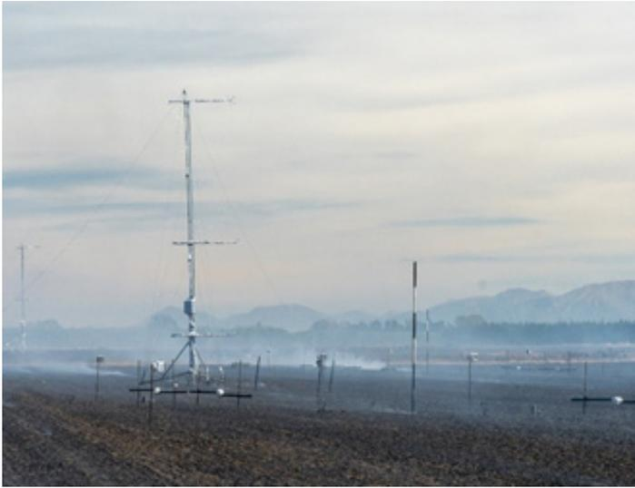
**Figure 3.** A post-burn view of one of Scion's 10m towers equipped with sonic anemometers to measure three-dimensional air movements, and thermocouples to record vertical flame and air temperatures, as the experimental fire moves by. A range of the US Forest Service team's equipment, including a flame height reference pole, in-fire cameras, heat flux and pressure sensors, and horizontal thermocouple arrays, can also be seen.
