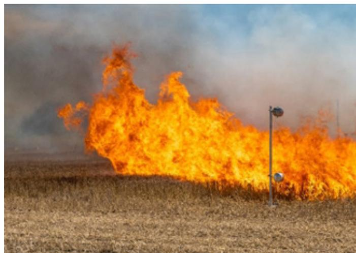
**Figure 2.** A stubble experimental fire moves past a set of "in-fire" video cameras being used to monitor flame front dynamics and fire spread rate.
