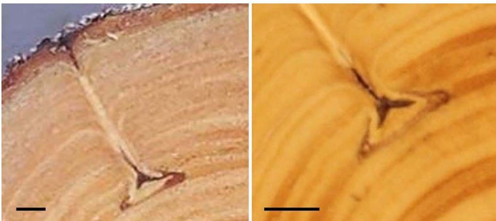
FIGURE 4: Increasing cambial damage and disruption of subsequent growth ring continuity are occlusion features normally associated with Type 2 pockets. These features are becoming evident in these two examples. Often there is a narrow, radial defect extending from the resin pocket to the bark. No evidence of resin blemishes (Bar = 10 mm).
