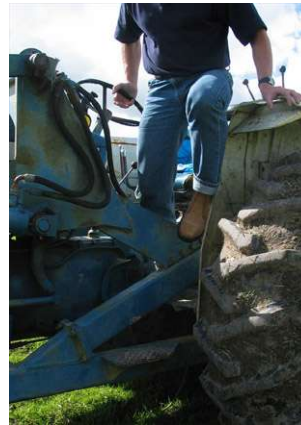
Figure 3. Trip hazards introduced where a fore-end loader has been added.
