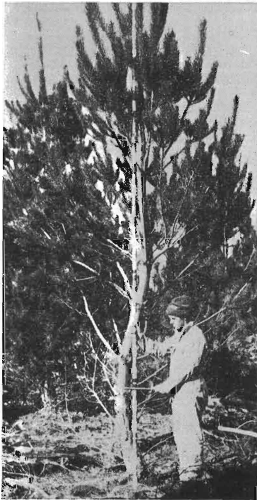
FIG. 5—Measuring sinuosity — the distance from the centre of the pole to the centre of the whorl represents the degree of sinuosity.
