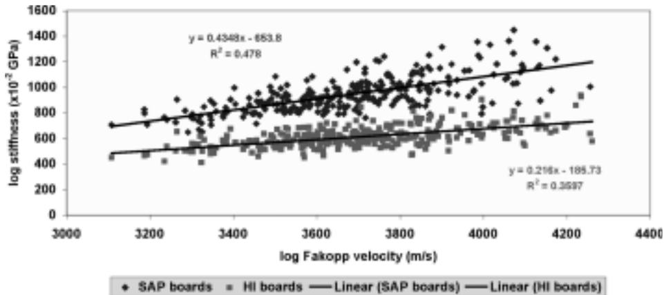
FIG. 3—Relationship between mean log stiffness (mean of all boards from each log) grouped into product type and log FAKOPP velocity, N=316.
