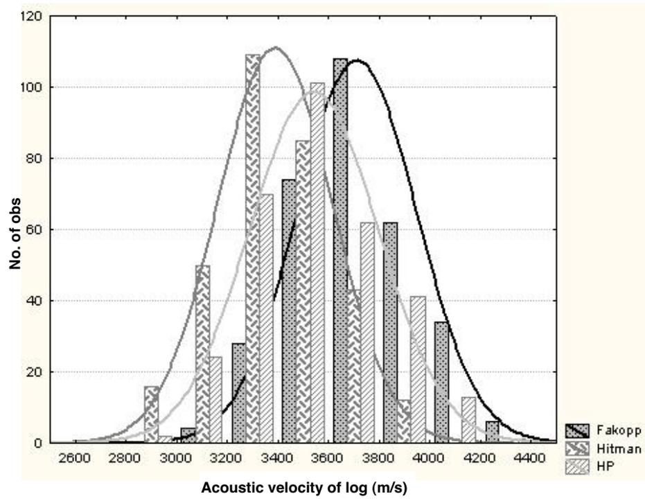
FIG. 2–Distribution of acoustic velocity for logs in the study according to the FAKOPP, Hitman, and HP measurements.
