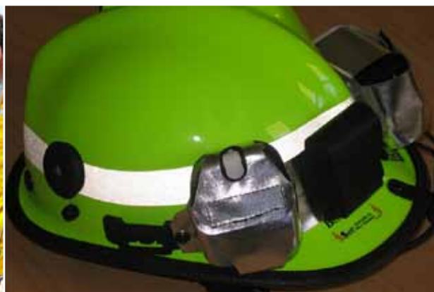
Figure 2. Modified helmet with sensors attached
