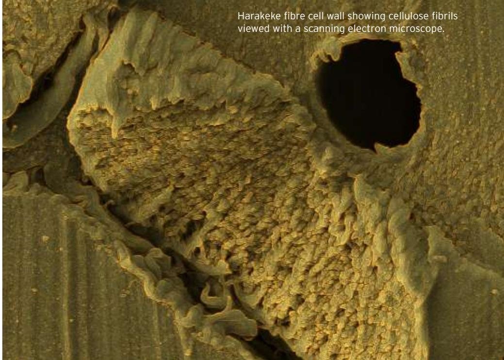
Harakeke fibre cell wall showing cellulose fibrils viewed with a scanning electron microscope.
