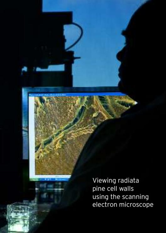
Viewing radiata pine cell walls using the scanning electron microscope
