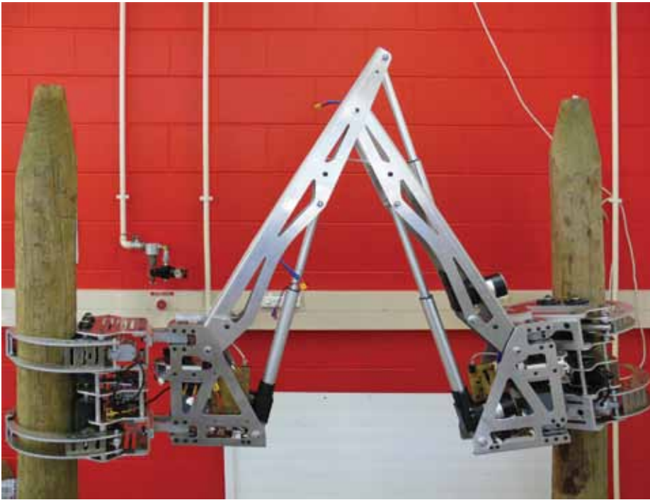
The tree-to-tree machine can move using trees as supports.
