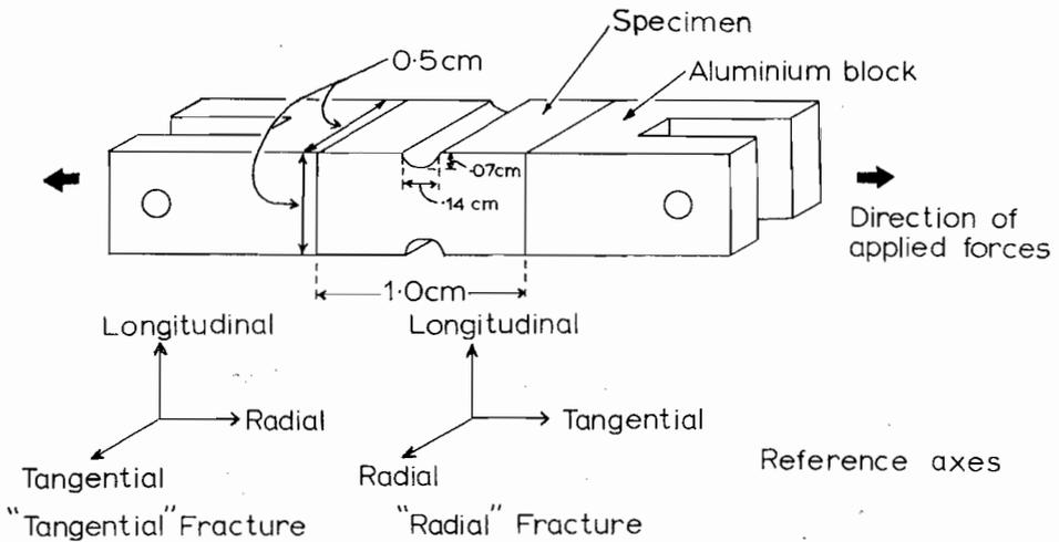
FIG. 2—Specimen shape and dimensions
