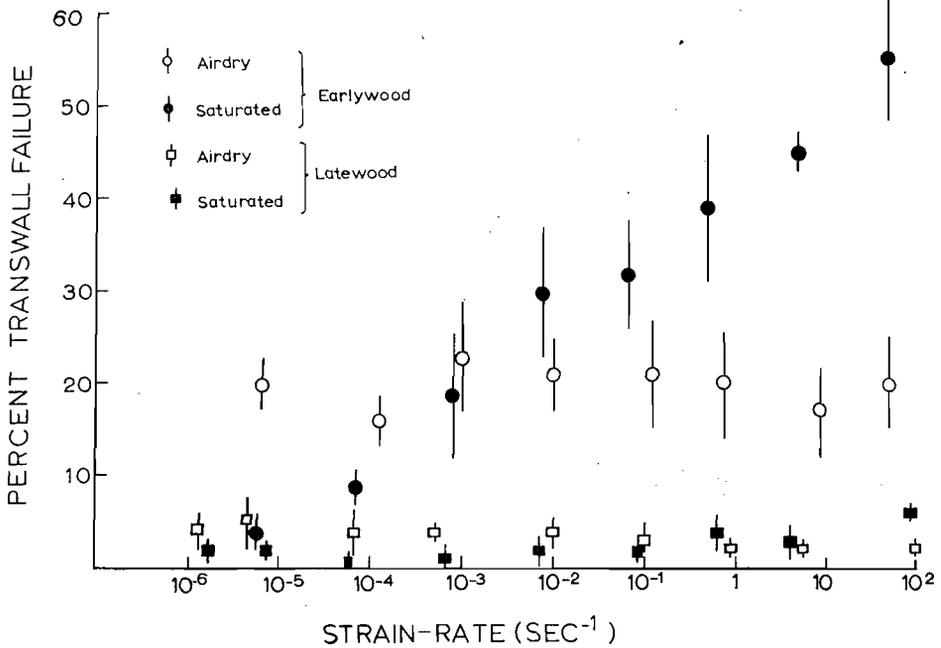
FIG. 9—Effects of strain-rate, moisture content and tracheid structure on the amount of transwall failure produced during the fracture of *Pinus radiata* by radial forces ...
