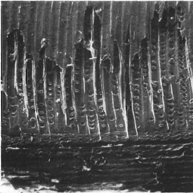
FIG. 5—Transwall failure produced by radial loading ( $\times 300$ )
