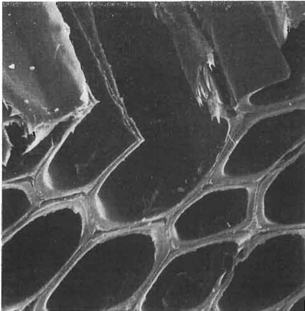
FIG. 8—Close up view of transwall failure ( $\times 2100$ )
