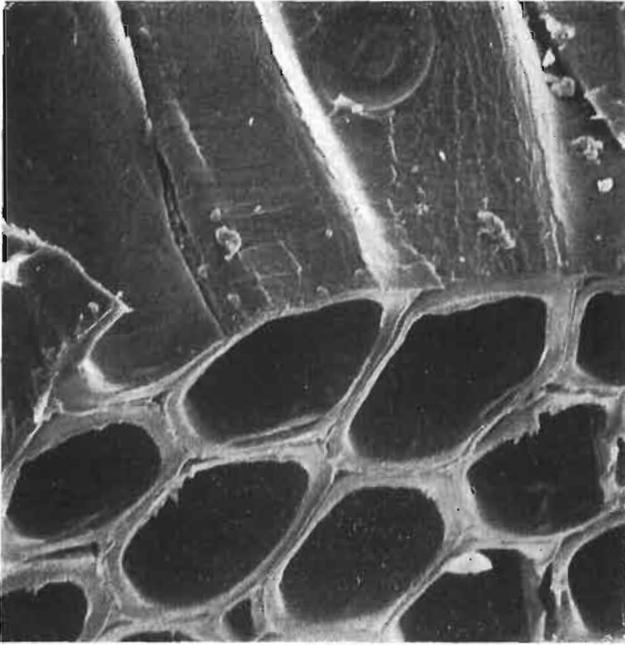
FIG. 4—Transwall and intrawall failure in earlywood ( $\times 2100$ )
