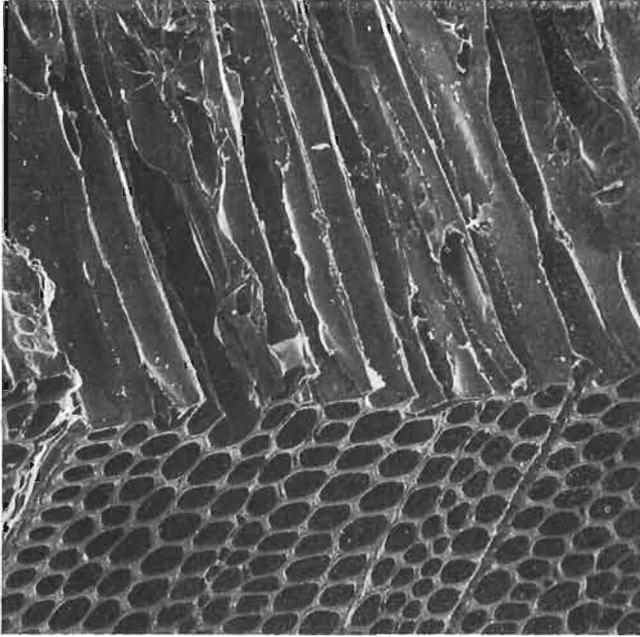
FIG. 7—Surface of an earlywood specimen broken while saturated at a strain-rate of  $10^2\text{sec}^{-1}$  ( $\times 420$ )
