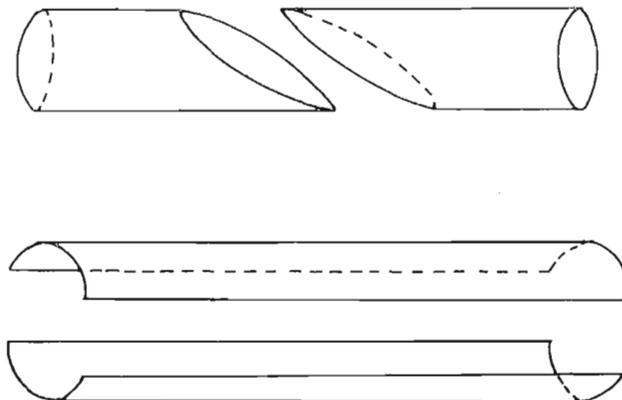
FIG. 6—(a) "Radial" transwall failure
