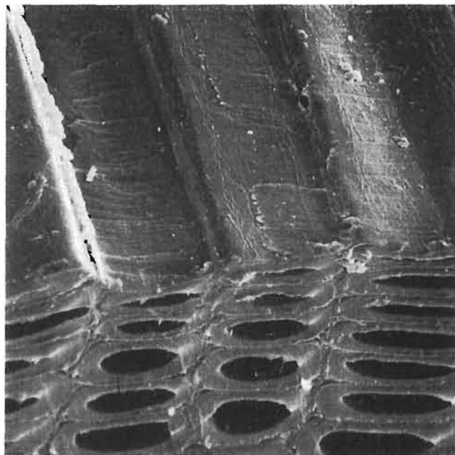
FIG. 3—Intrawall failure in latewood ( $\times 2200$ )
