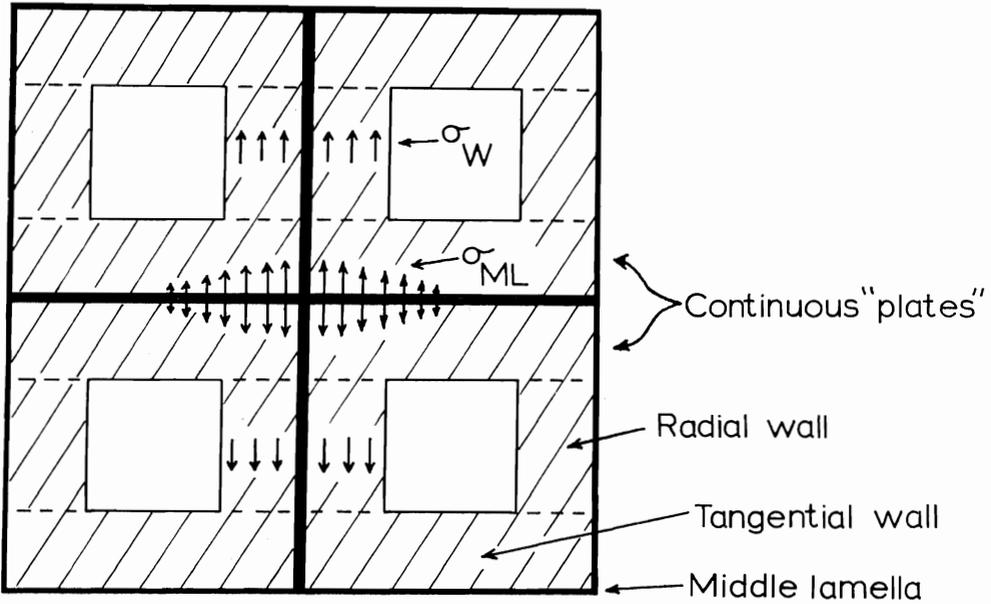
FIG. 10—Perfectly aligned latewood tracheids showing wall ( $\sigma_W$ ) and middle lamella ( $\sigma_{ML}$ ) stresses.
