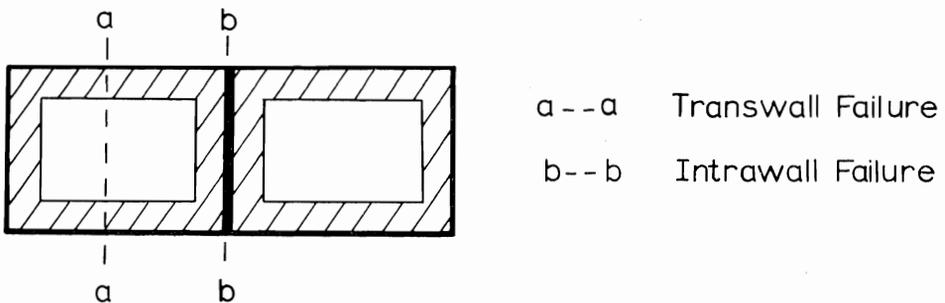
FIG. 1—Transwall and intrawall failure
