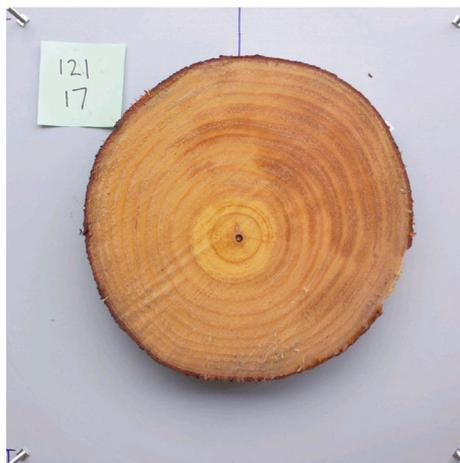
FIG. 2—Image of sample disc 121/17 corrected for perspective distortion using a two-dimensional projective transform.
