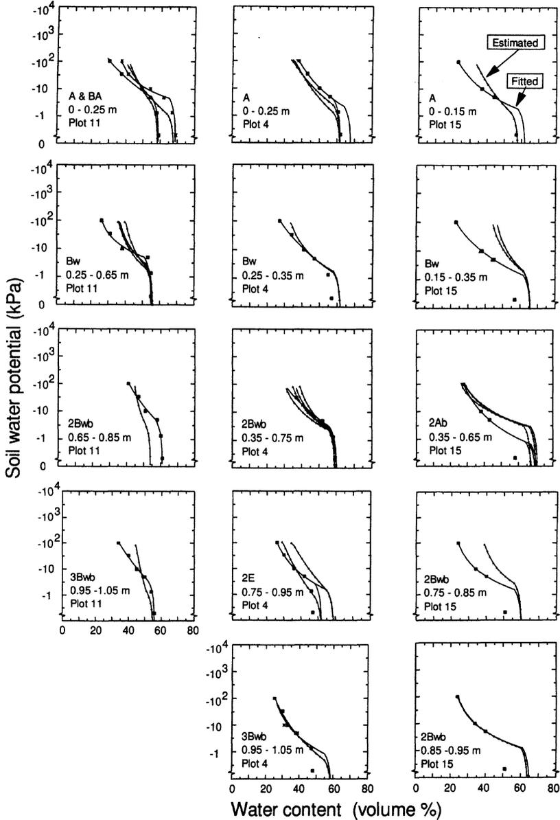
FIG. 3—Soil water retention curves fitted to values measured in the laboratory (fitted) and soil water retention curves estimated through comparison of model output with soil water contents measured in field (optimal parameter sets, estimated). Symbols represent values measured in the laboratory. The measured data points and fitted curves represent individual horizons, whereas estimated curves represent 0.1-m depth intervals.
