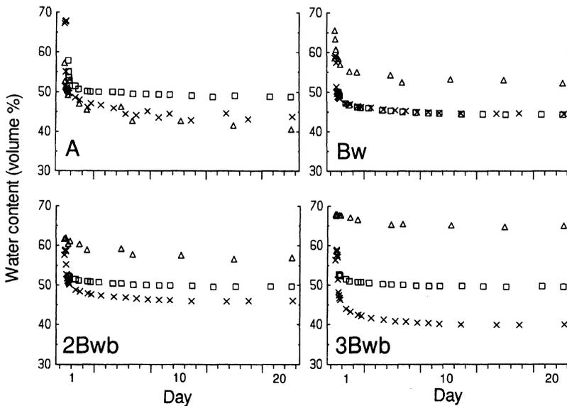
FIG. 1—Measured soil water content in the four horizons during drainage. Crosses represent Plot 4, squares Plot 11 and triangles Plot 15.
