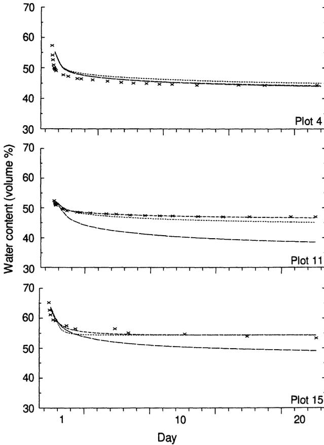
FIG. 2—Simulated (lines) and measured (crosses) soil water contents for the uppermost 1-m layer during drainage. Simulated values are represented by long dashed line for laboratory parameter set, medium dashed line for optimal parameter set, and short dashed line for common parameter set.
