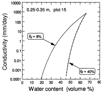
FIG. 4—Illustration of the effect of  $\theta_r$  on the hydraulic conductivity curves.
