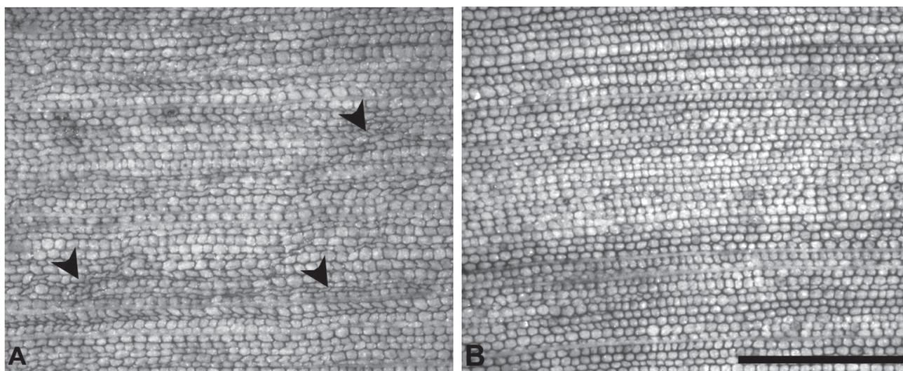
FIGURE 2: (A) Severely checked wood sample. The arrowheads indicate the presence of collapsed cell files; (B) Non-checked sample; Scale bar = 5cm.
