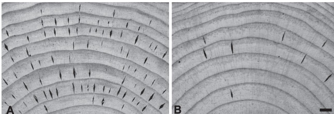
FIGURE 1: (A) Severely checked disk displaying a large number of growth rings with checks. More checks were seen in each new growth ring affected;
