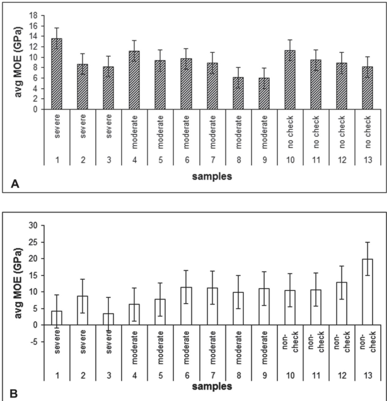
FIGURE 3: MOE data analysis of the checked and non-checked wood samples.
