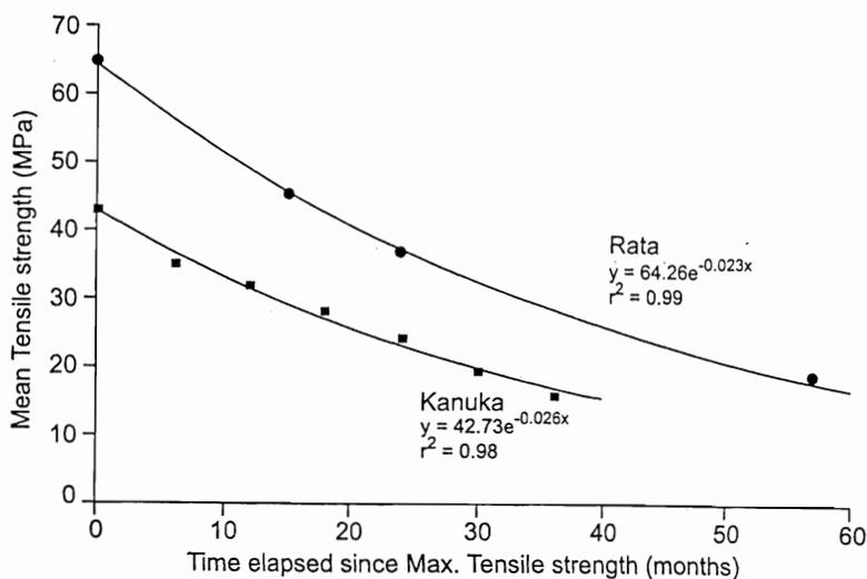
FIG. 3—Root-wood strength decline curves. Negative exponential relationship between mean tensile strength (MPa) and time elapsed since occurrence of maximum tensile strength (months) for root-wood of kanuka and southern rata.
