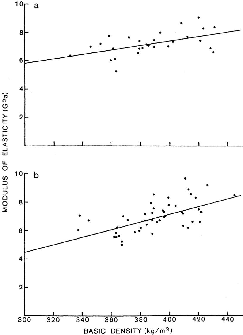
FIG. 3—Mean modulus of elasticity as a joist (EJ) v. basic density of log (BD) for (a) 100 x 50-mm and (b) 200 x 50-mm material.
