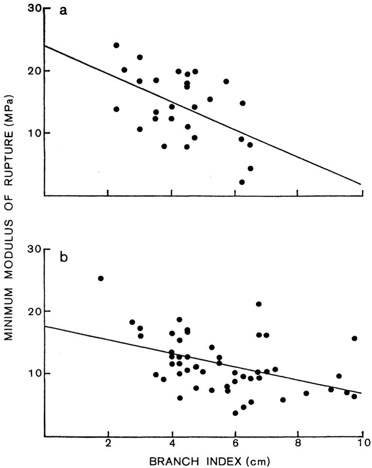
FIG. 4—Minimum modulus of rupture (MINRJ) v. branch index (BI) for (a) 100 × 50-mm and (b) 200 × 50-mm material.
