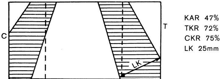
FIG. 2—Sample knot diagram. KAR = knot area ratio; TKR = tension margin knot area ratio; CKR = compression margin knot area ratio; LK = largest knot.
