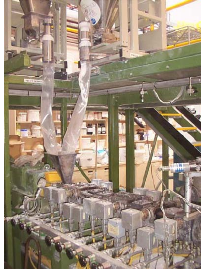
Production at 20-800kg/hour on D=83mm
