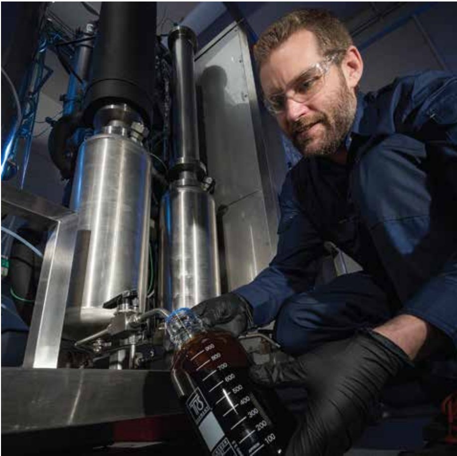
Technician Ben McDonald collecting bio-oil from Scion's fast pyrolysis plant.
