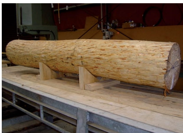
FIGURE 3: Log 1 (pruned) on carriage awaiting scanning
