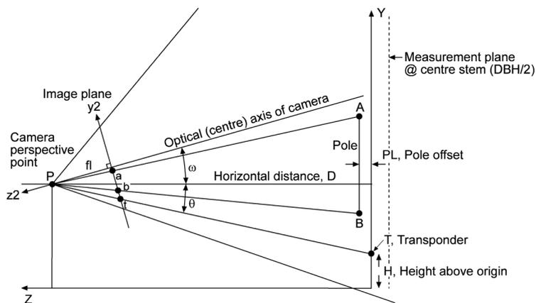
FIG. 1—The TreeD camera-to-tree geometry
