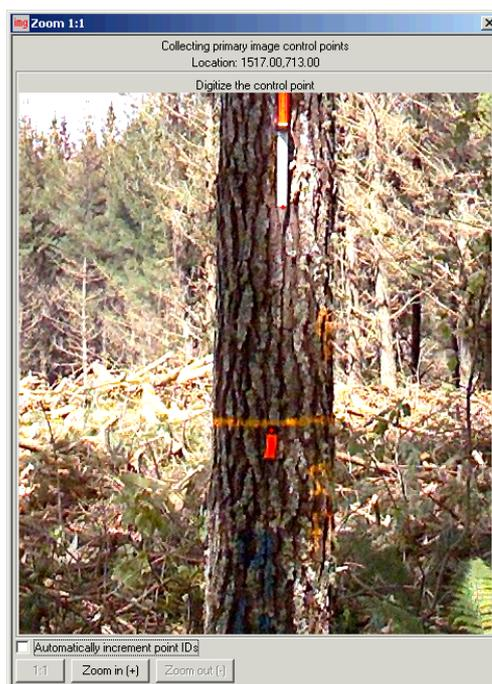
FIG. 3—The digitising window. This example shows the bottom of the height pole and the transponder digitised.
