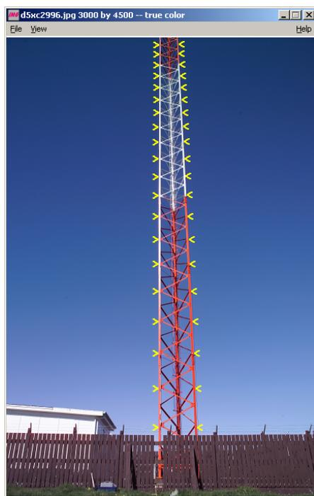
FIG. 4—An image of the radio mast showing the location of some of the points used to assess the accuracy of TreeD.
