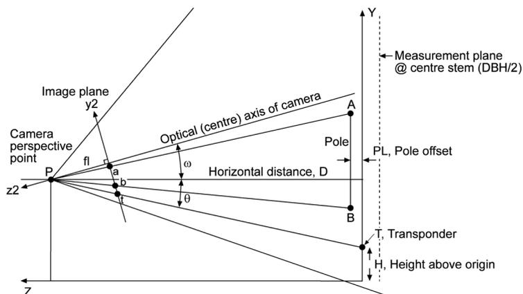
FIG. 1—The TreeD camera-to-tree geometry
