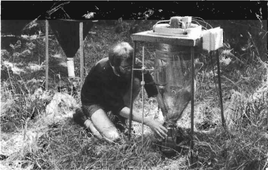
FIG. 1—Plastic cone frass trap with collecting tube in background. Suction trap, complete with isopropyl alcohol reservoir, being serviced in foreground.
