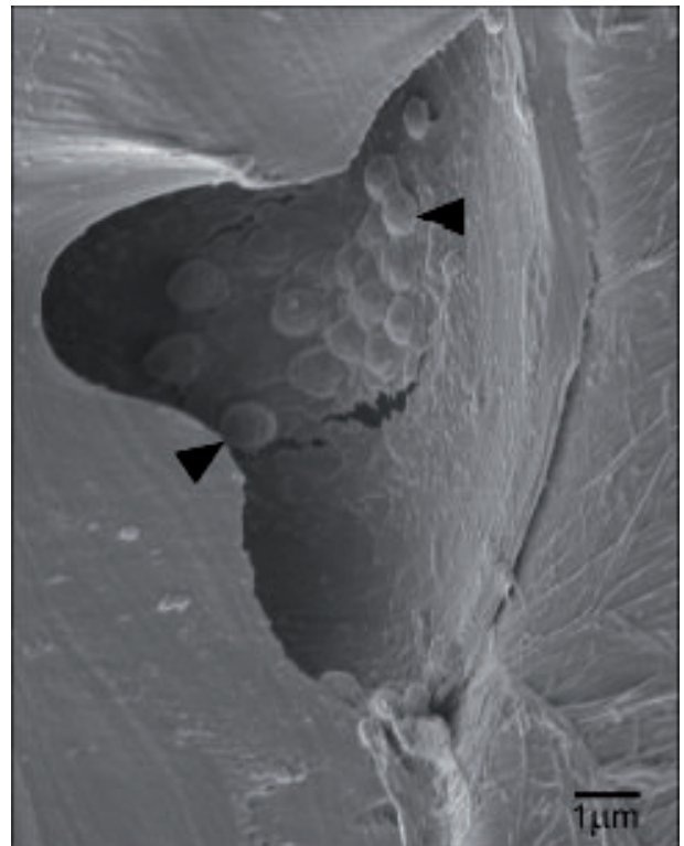
FIGURE 7: Section from ponded wood showing bacteria associated with a pit membrane (arrowheads), which is perforated. FE-SEM micrograph.
