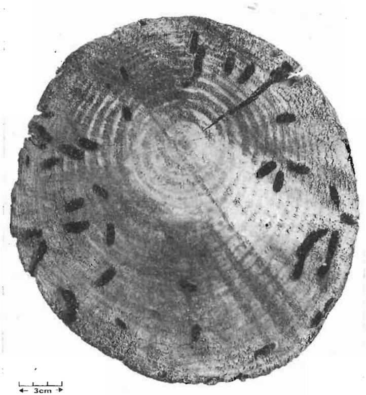
FIG. 5—Damage to log 12 months after first attack.
