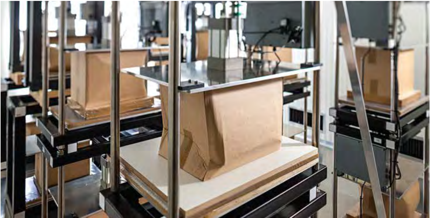
Scion's WHITE room can test up to 25 corrugated boxes under accelerated conditions.
