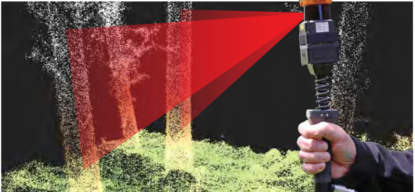
The hand held scanner provides highly detailed 3D data of individual trees within a stand where GPS is unavailable.
