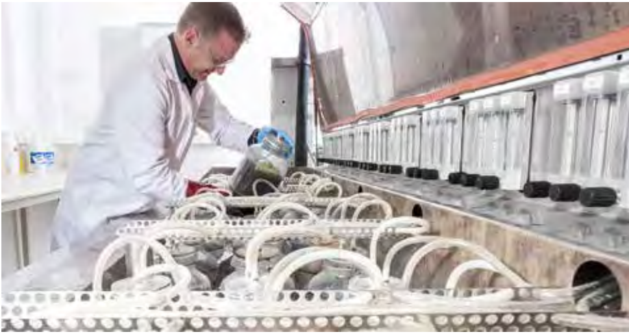
Scion's biodegradation facility measures and quantifies the aerobic composting of materials.
