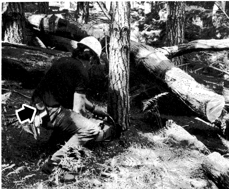
FIG. 5—Cutter wearing activity recorder (Mk II) on belt whilst working in P. radiata at Tumut.
