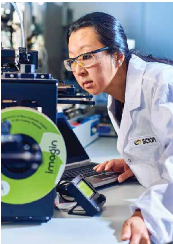
Project leader Dr Marie Joo Le Guen observes the Imagin Plastics wood-fill filament as the 3D printer prints a sample piece.
