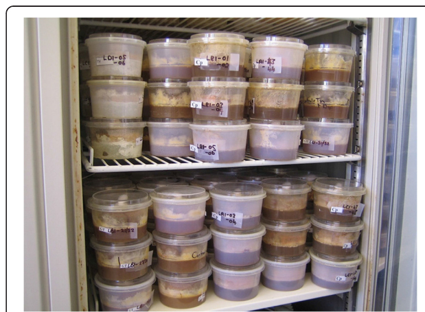
Figure 1 Decay testing of the coast redwood heartwood blocks, and the radiata pine sapwood control blocks, with fungal cultures in an incubator.
