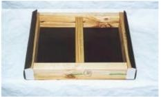
Using these methods Scion was able to test seven timber treatment options in a relatively short time, including the three approved treatment methods, to determine which conferred framing timber resistance before, during and after construction. The primary objective of the "after
