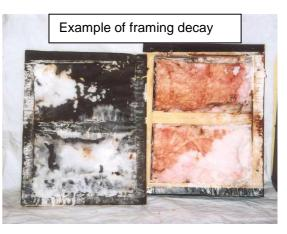
resistance to decay for periods sufficient for leaks to be detected and rectified (potentially for up to 10 years).
