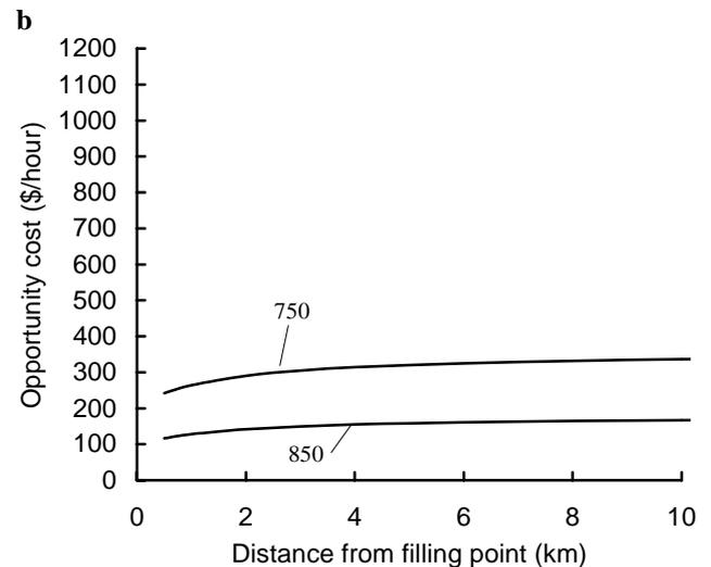
**Figures 4. (a)** The differences in delivery rate from a B2 Squirrel for a range of bucket sizes; and **(b)** the opportunity cost of using a 750 and 850 litre bucket instead of a 950 litre one.
