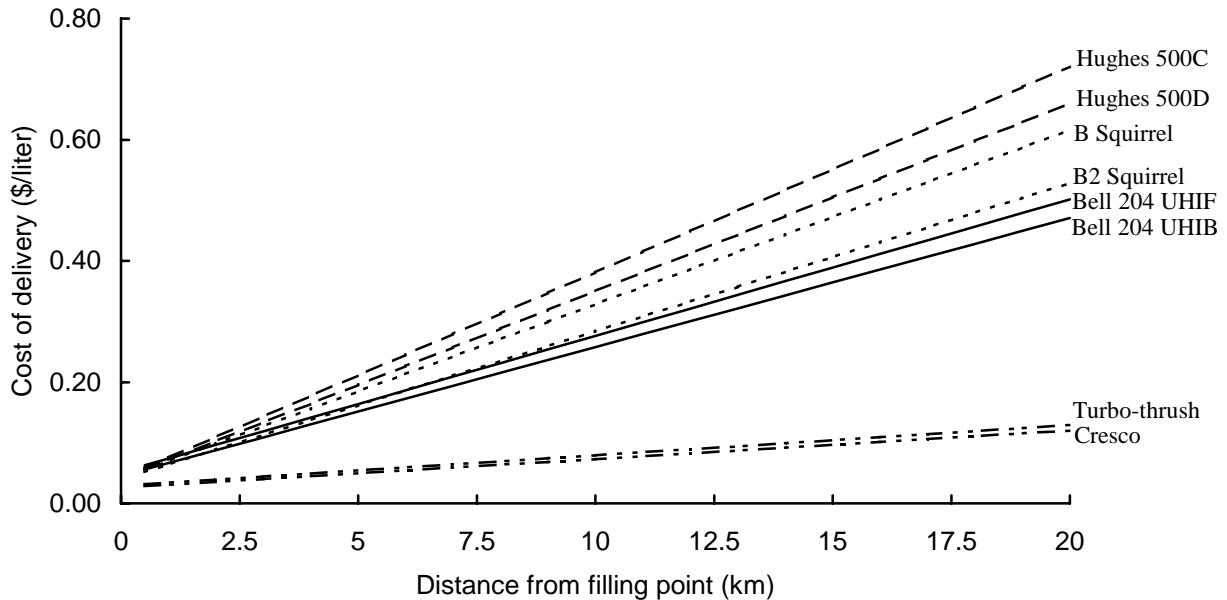
**Figure 2.** Comparison of the cost of water delivery per litre for selected fixed-wing and rotary-blade aircraft operating from a range of distances between the fire and the filling point.
