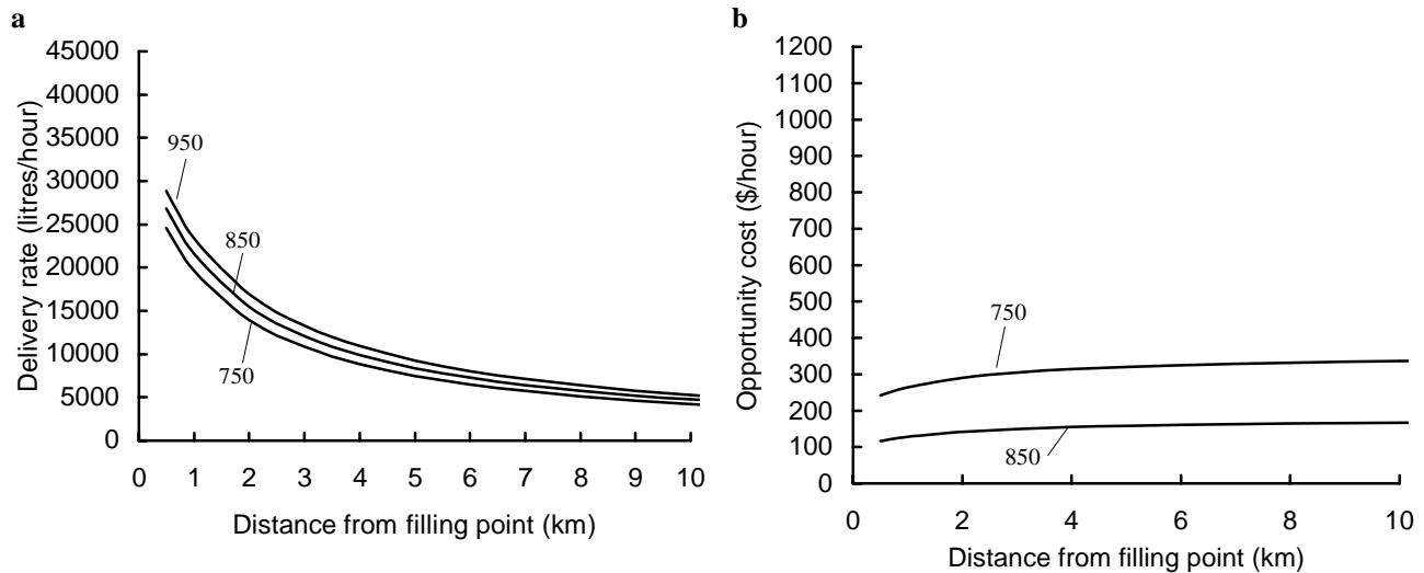
**Figures 4.** (a) The differences in delivery rate from a B2 Squirrel for a range of bucket sizes; and (b) the opportunity cost of using a 750 and 850 litre bucket instead of a 950 litre one.
