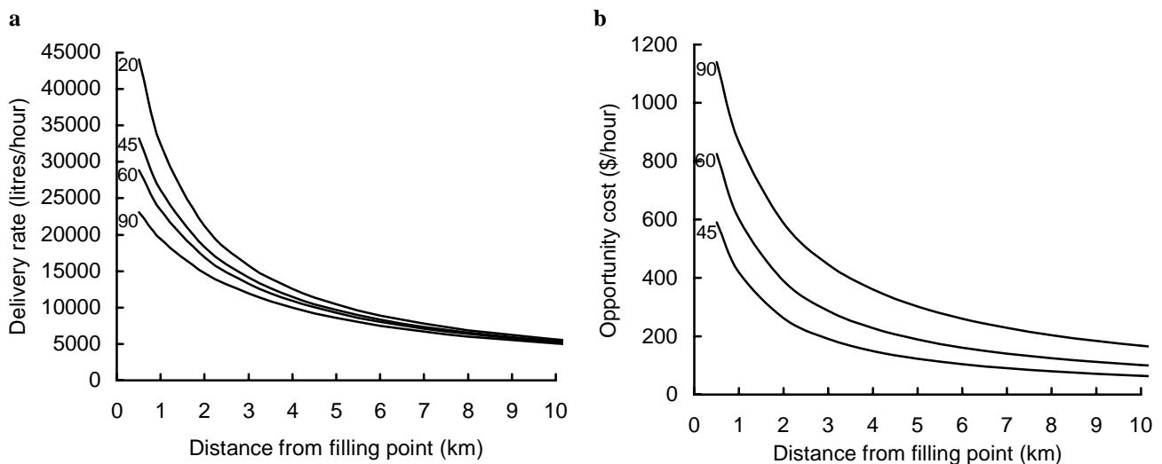
**Figures 3.** (a) The differences in delivery rate from a B2 Squirrel for a range of filling times; and (b) the opportunity cost of 45, 60 and 90 second filling when compared to a 20 second fill.
