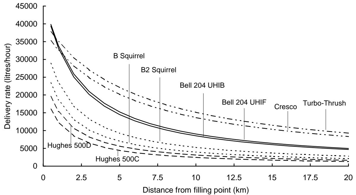
**Figure 1.** Comparison of the rate of water delivery per hour for selected fixed-wing and rotary-blade aircraft operating from a range of distances between the fire and the filling point.
