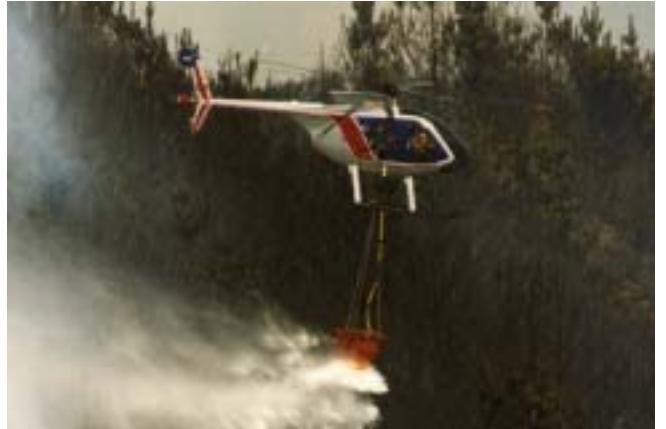
The scenario assumes that all filling is done using a pump with an output of 1400 litres per minute. Positioning and acceleration add 20 seconds to a helicopter refill, while landing, and positioning add 1 minute to an aeroplane refill.
