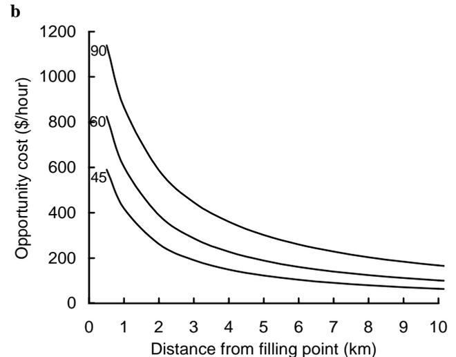
**Figures 3. (a)** The differences in delivery rate from a B2 Squirrel for a range of filling times; and **(b)** the opportunity cost of 45, 60 and 90 second filling when compared to a 20 second fill.
