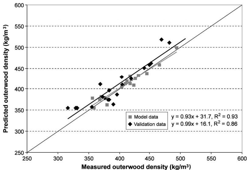
FIG. 7—Performance of the national wood density model for *P. radiata* based on the model outerwood density data and the validation data.
