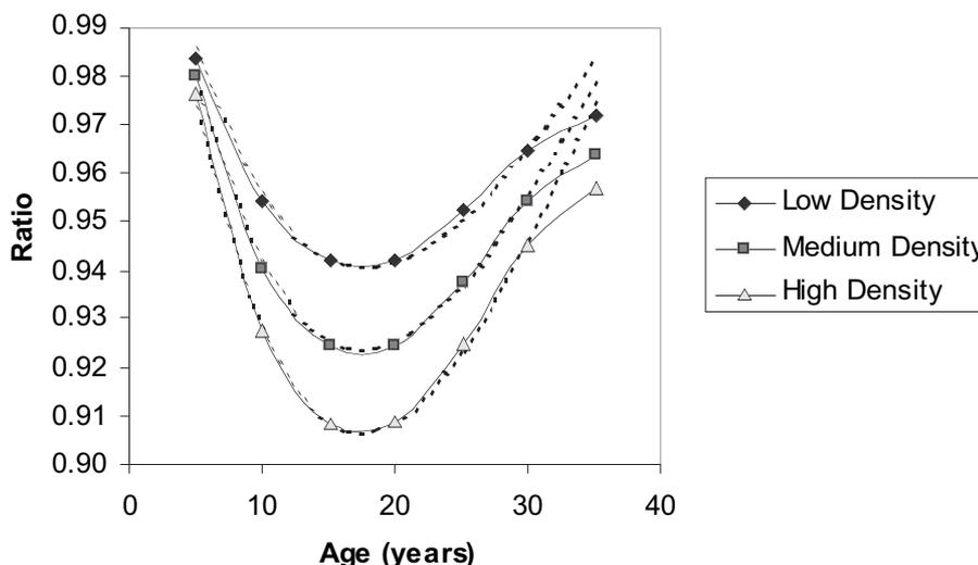
FIG. 6—Ratios of growth sheath to breast-height ring density estimated for rings formed at a range of ages on low-, medium-, and high-density sites. The dashed lines were obtained using Equation (6).
