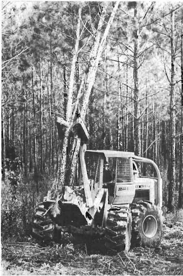
FIG. 2—An accumulator-type felling head attached by a one-plane mounting to a wheeled loader.
