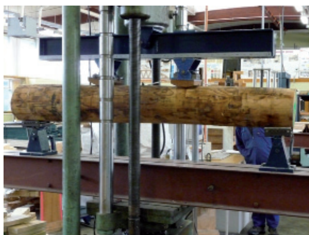
FIGURE 1: A pole under test in bending
