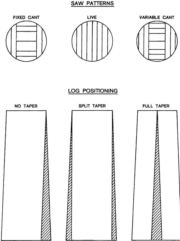
FIG. 1—Sawing procedures.
