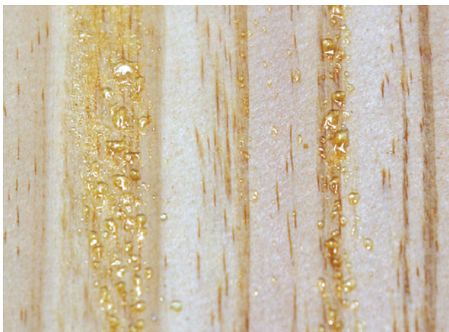
Figure 3. Heavy resin bleed
