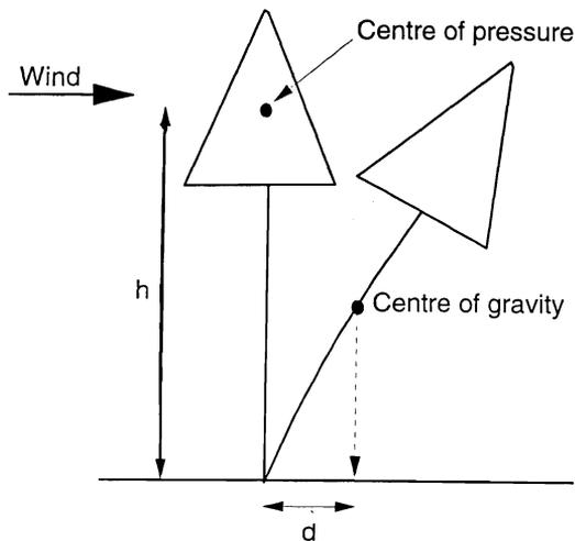
FIG. 1—The two components of the overturning moment acting on a tree. The first component is due to the wind acting at the centre of pressure of the tree crown at height  $h$ . Once the tree has deflected, the weight of the offset stem plus crown, acting over the lever arm  $d$ , provides the second component (from Quine *et al.* 1995).
