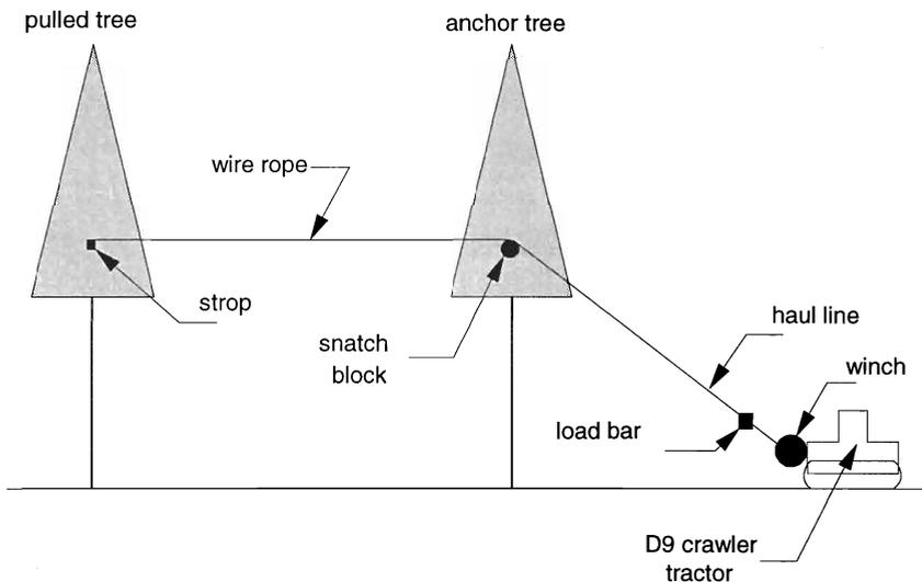
FIG. 2—Schematic diagram of the tree winching system.
