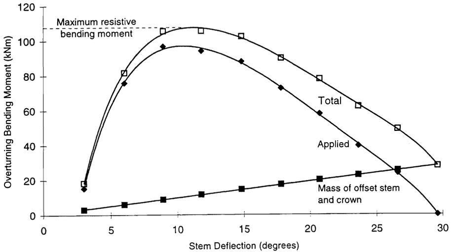
FIG. 4—The relative contribution of the applied bending moment and the bending moment due to the offset mass of the tree to the total overturning bending moment at various angles of stem deflection.
