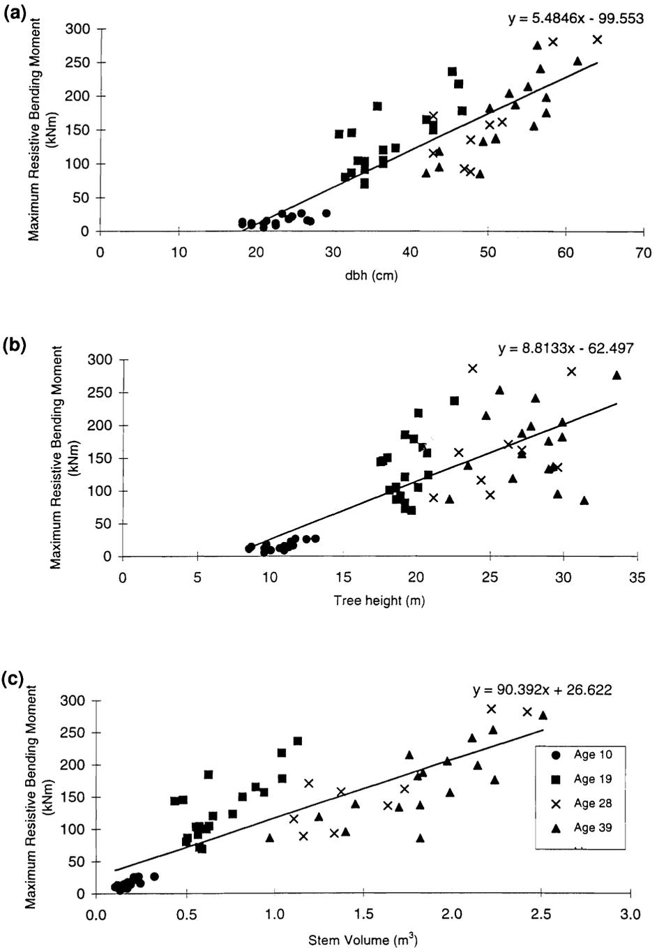
FIG. 6—Relationships between maximum resistive bending moment and (a) diameter at breast height, (b) tree height, and (c) stem volume.
