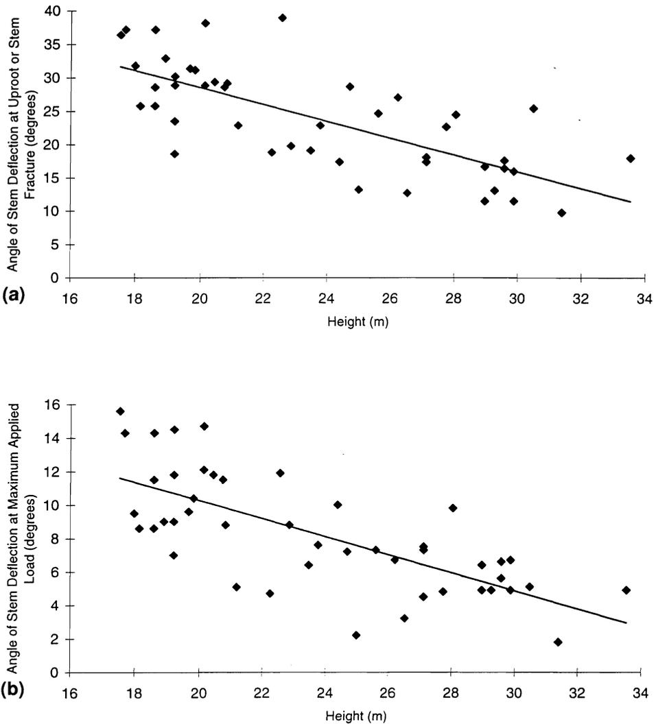
FIG. 5—Relationships between tree height and (a) the angle of stem deflection at uproot or stem fracture, and (b) the angle at the point of maximum applied moment.
