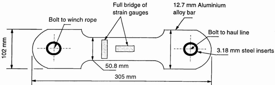
FIG. 3—Dimensions of the strain bar used to measure load on the winch rope.
