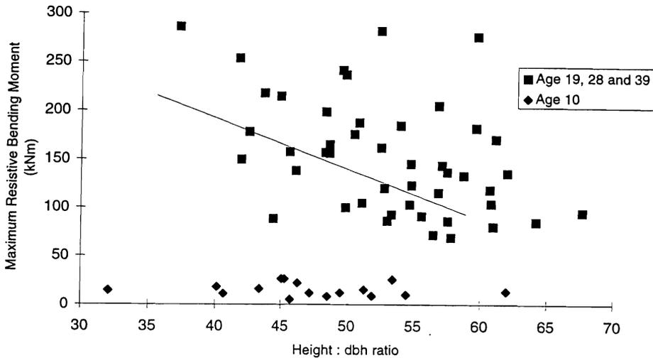
FIG. 7—Relationship between stem taper (height : dbh ratio) and maximum resistive bending moment.
