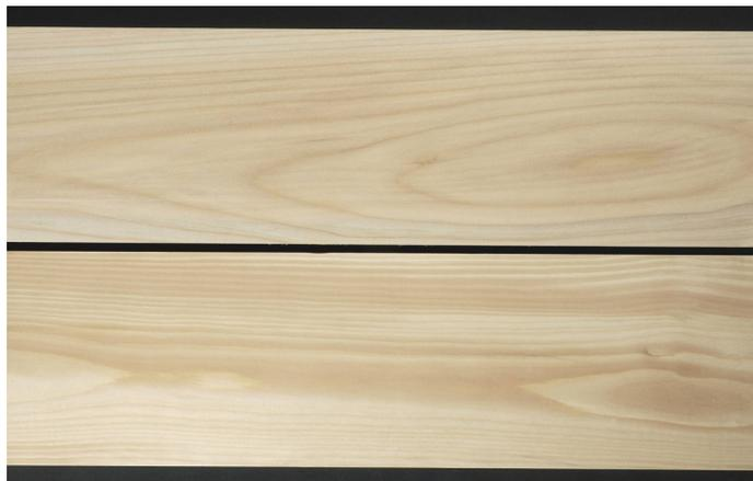
FIG. 3—Cut and planed sapwood boards (150 × 50 mm) from plantation-grown kauri.
