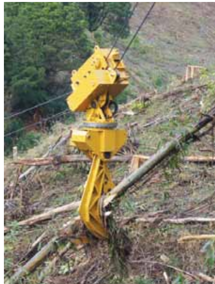
The hydraulic-based hauler grapple.
