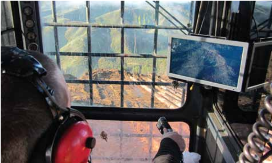
The CutoverCam emits high frequency video of ground operations back to the hauler operator.
