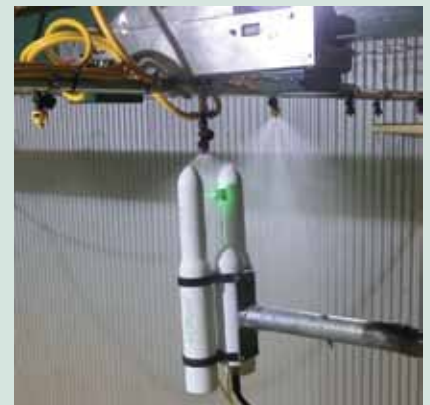
Measuring spray droplets.
