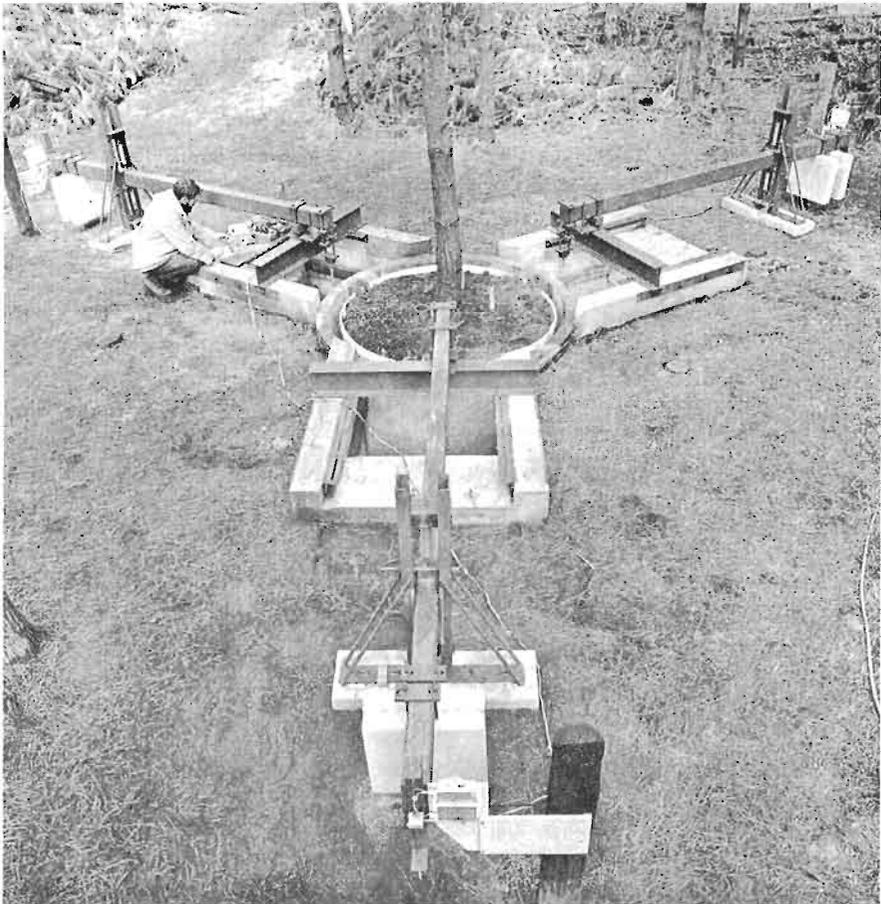
FIG. 2—View of complete lysimeter in operation.
