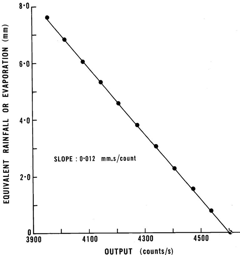
FIG. 3—Calibration of a lysimeter.
