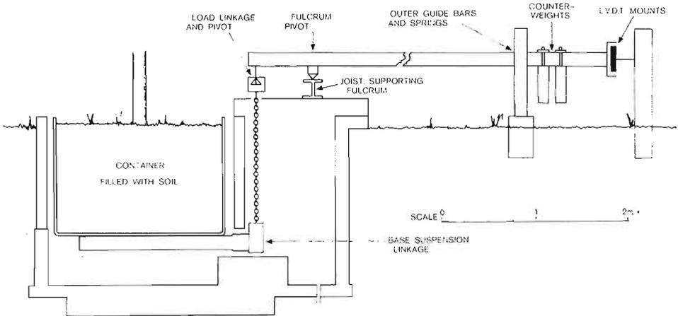
FIG. 1—Cross-section through lysimeter container and one beam and fittings, showing location of main components.
