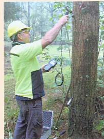
Measuring timber stiffness on a standing tree using the IML meter.
