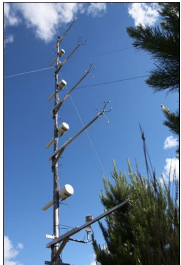
10 m tower arrayed with sensors to measure wind and temperature every second or less.
