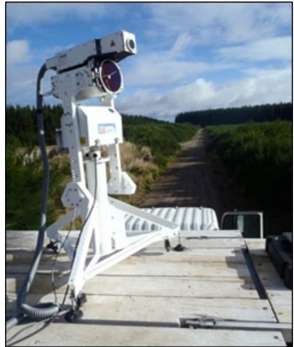
University of South Carolina's backscatter LiDAR measures the spray drift aerosol cloud.
