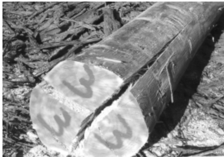
FIG. 4—End-splitting in peeler log (left) and sawlog (below) of Tree 24.
