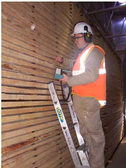
Testing airflow in a kiln.
