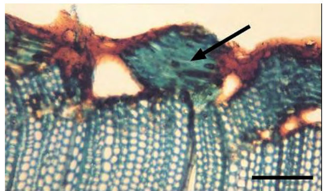
Figure 1. Light micrograph showing greatly distorted surface tissue masses and associated large cracks. The distorted tissues appear fuzzy and are not clearly resolved (arrow). Bar = 200 \mu\text{m} .
