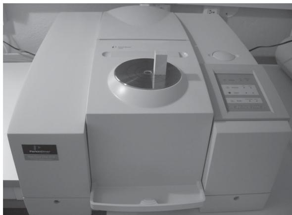
FIG. 1—The PerkinElmer Spectrum One NTS system. The wood specimen was placed with a cross-sectional surface on the circular window over the light source.
