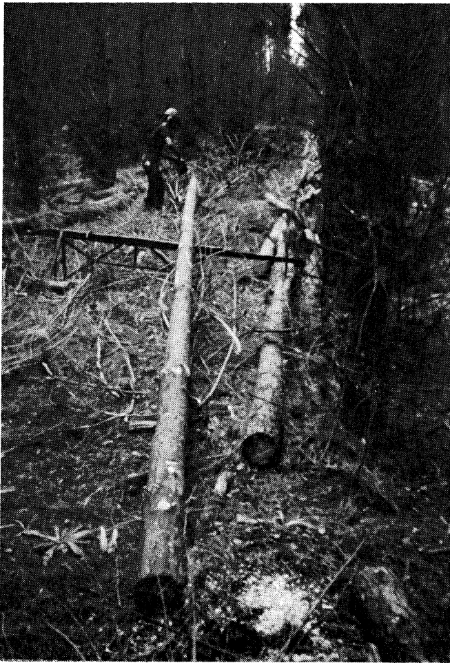
FIG. 4—Felled tree across felling bench being trimmed before sliding into wood zone
