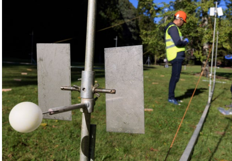
Staff preparing the first trial which used collectors, placed through canopy and on the ground, to capture how deeply the dye penetrated and drifted.
