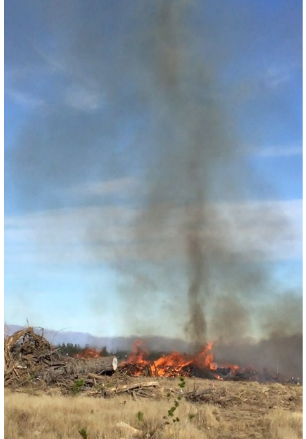
The research in Twizel successfully generated fire whirls in the field – a world first at this scale. After igniting the slash pile 20 metres in diameter, the research team was able to generate a 'smoke devil' that took up the flame and generated a fire whirl.
