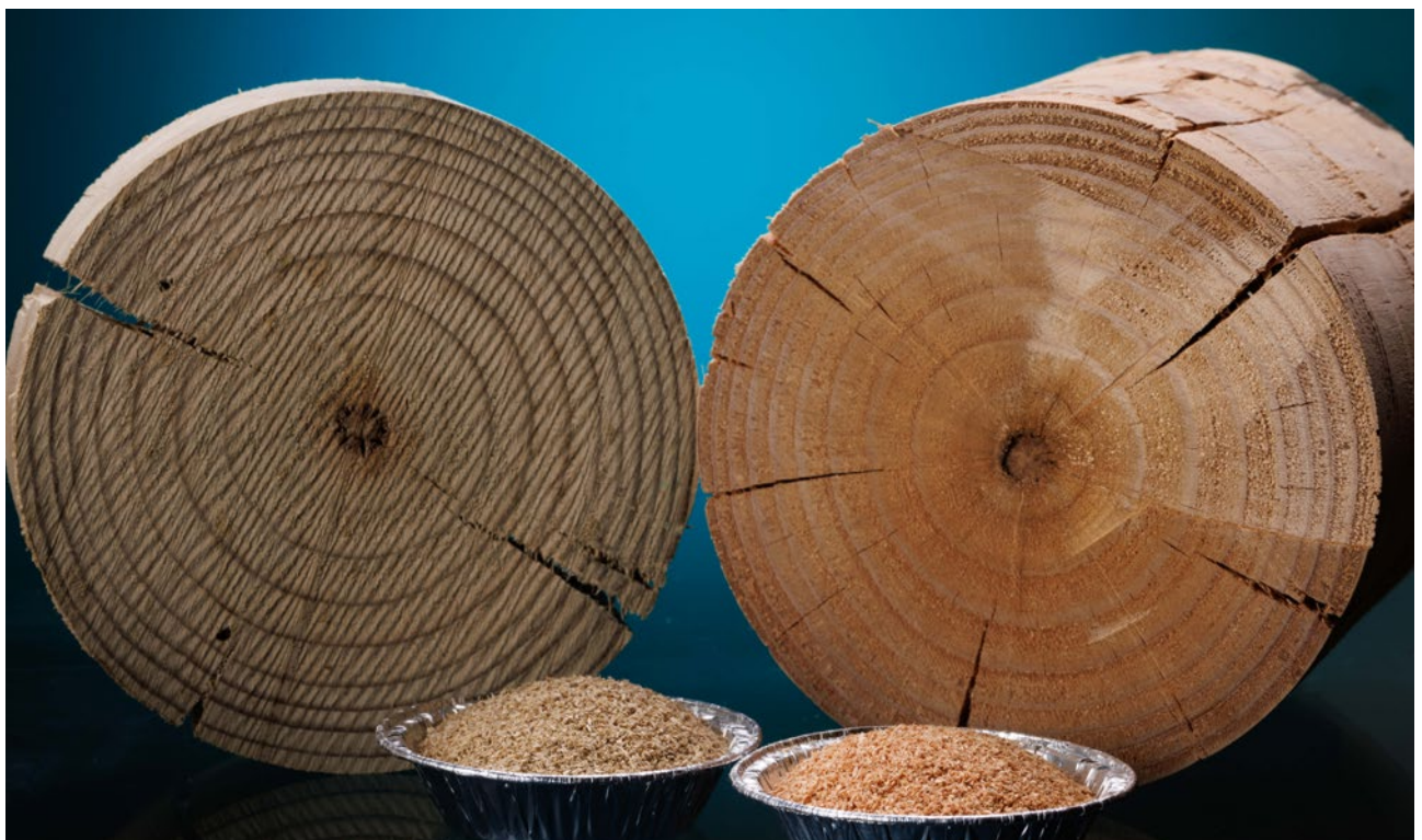
The CCA treated timber, right, can be remediated to keep it in the circular bioeconomy.
