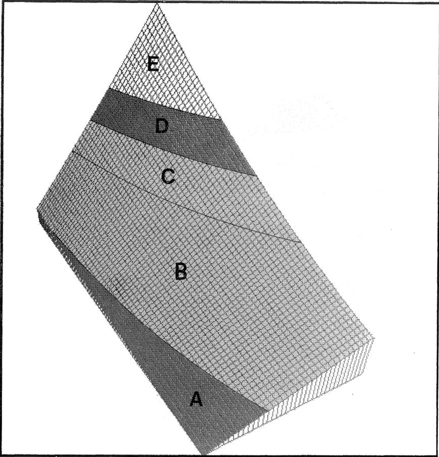
FIG. 1—Moisture content reduction surface during platen pressing of *Pinus radiata*: effect of changes in initial moisture content and strain.
