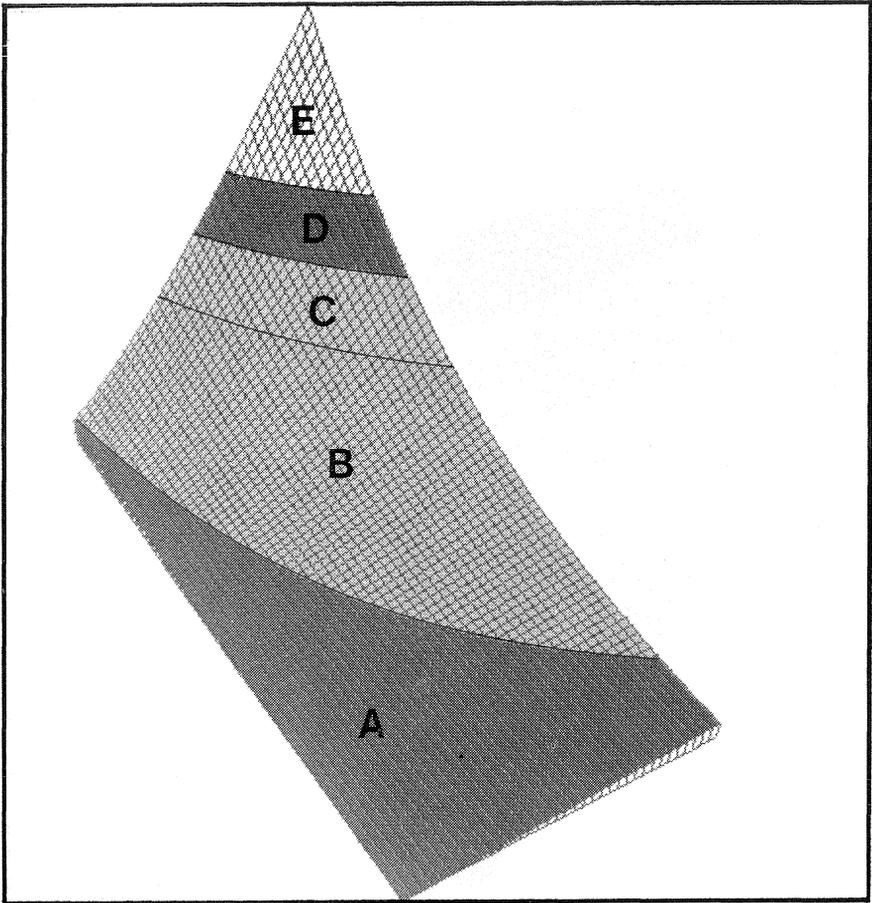
FIG. 2—Moisture content reduction surface during platen pressing of *Eucalyptus regnans*: effect of changes in initial moisture content and strain.
