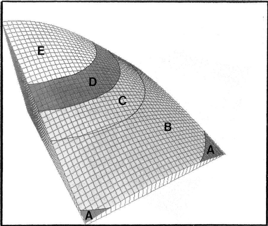
FIG. 3—Energy ratio surface during platen pressing of *Pinus radiata*: effect of changes in initial degree of pore saturation and strain.
